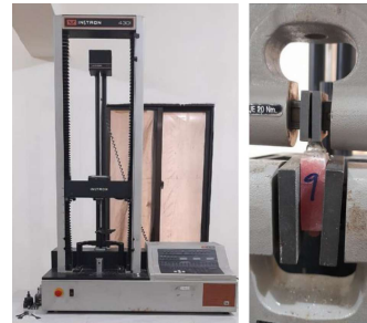
Step 9: Prepared assembly mounted on the Universal Testing Machine (INSTRON-4301)
